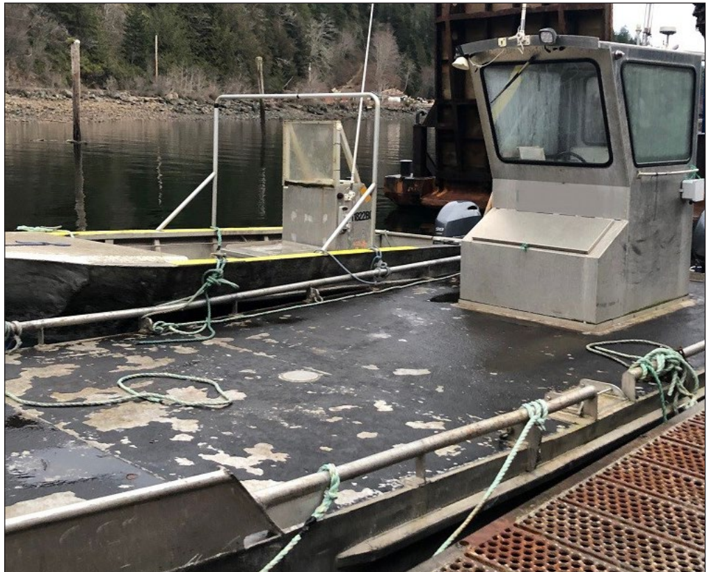
This flat deck boat pictured has structural damage below the deck, making it unsafe and unstable for farm use any longer.
